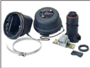
**DL/FAK and ZL/FAK Indicating Light Kits** are designed to provide visual indication of an energized heating circuit. The kit may be utilized as a power connection or an end termination kit. (PETK/SCTK termination kit required, order separately).
