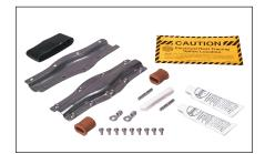
**SK-SX-OJ...**Ex e approved under-the-insulation repair and splice kit for overjacketed SX cables. Kit includes stainless steel shells, screws, grommets, RTV adhesive/sealant, insulation tape and the necessary wire pins/lugs.
